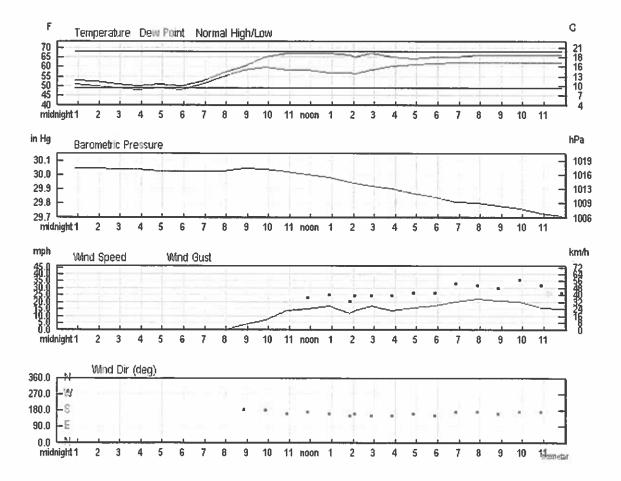
With sustained winds of 10 m.p.h. or higher for 13 hours, this day should have been one of our best producing energy days. When the data was downloaded at 11a.m. on September 19th, the software system was reporting energy production of -.09 kwh produced for September 18th. It also reported 2.74 kwh of energy produced for September 19th, in just the first 11 hours of that day.
